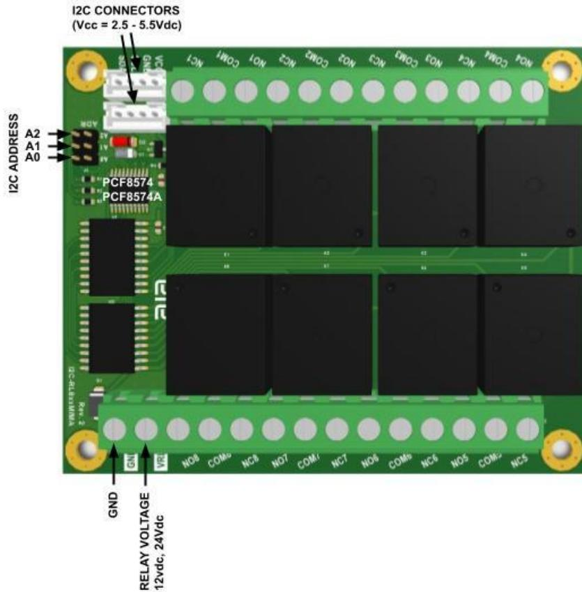
Figure 1: Board diagram
