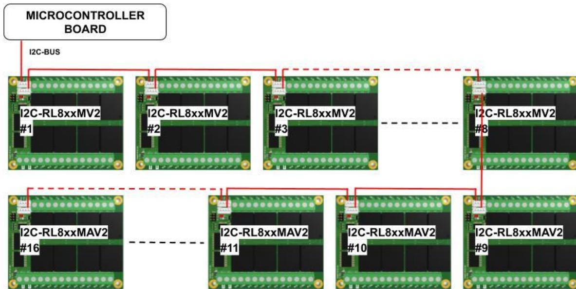
Figure 5: Multiple boards on a single bus
