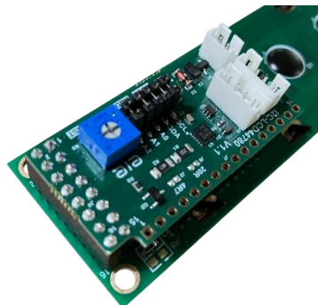
Figure 12: Install on a dual-line 8x2 pins connector
