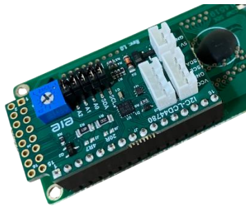
Figure 11: Install on a single-line 16 pins connector
